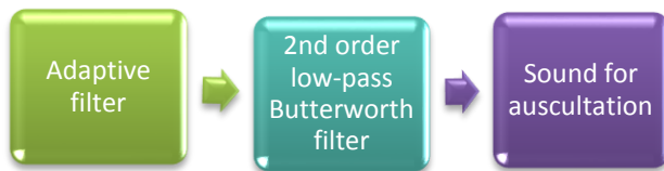
Fig. 12 The functional block diagram for improving the auscultation.
